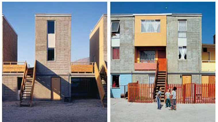
Fig. 8 : Elevation with and without extension ( Elemantal, 2005)
