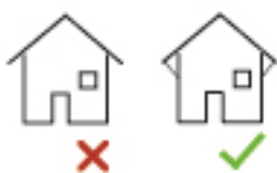
Figure 12; Anchor roof overhang to the wall
