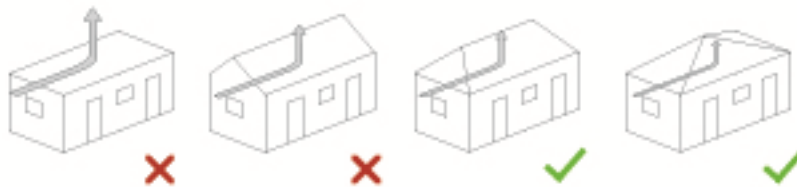
Figure 11; A flat roof and a gabled roof creates a stronger uplifting force than a hipped or pyramidal roof
