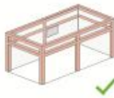
Figure 8b; Reinforced concrete frame with masonry infill
