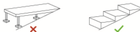
Figure 3; A big building should have a foundation divided in different levels when built in a slope.
