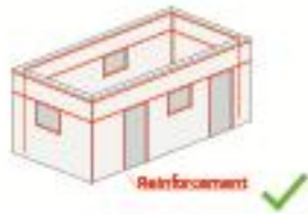
Figure 8a; Reinforcement marked in red
