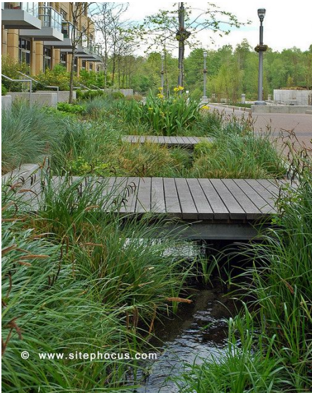
Open stormwater canals/wetlands
