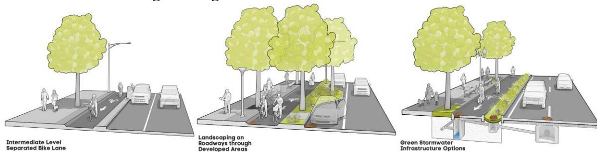
Figure 15 Various configurations of separated bike lanes (MassDOT, 2015)
