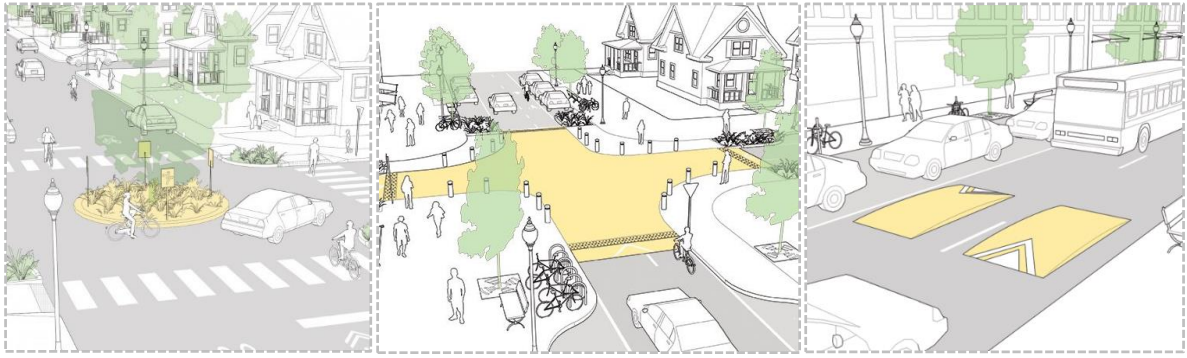
Figure 18 Roundabout, Raised intersection, Speed Cushion (NACTO, 2013)
