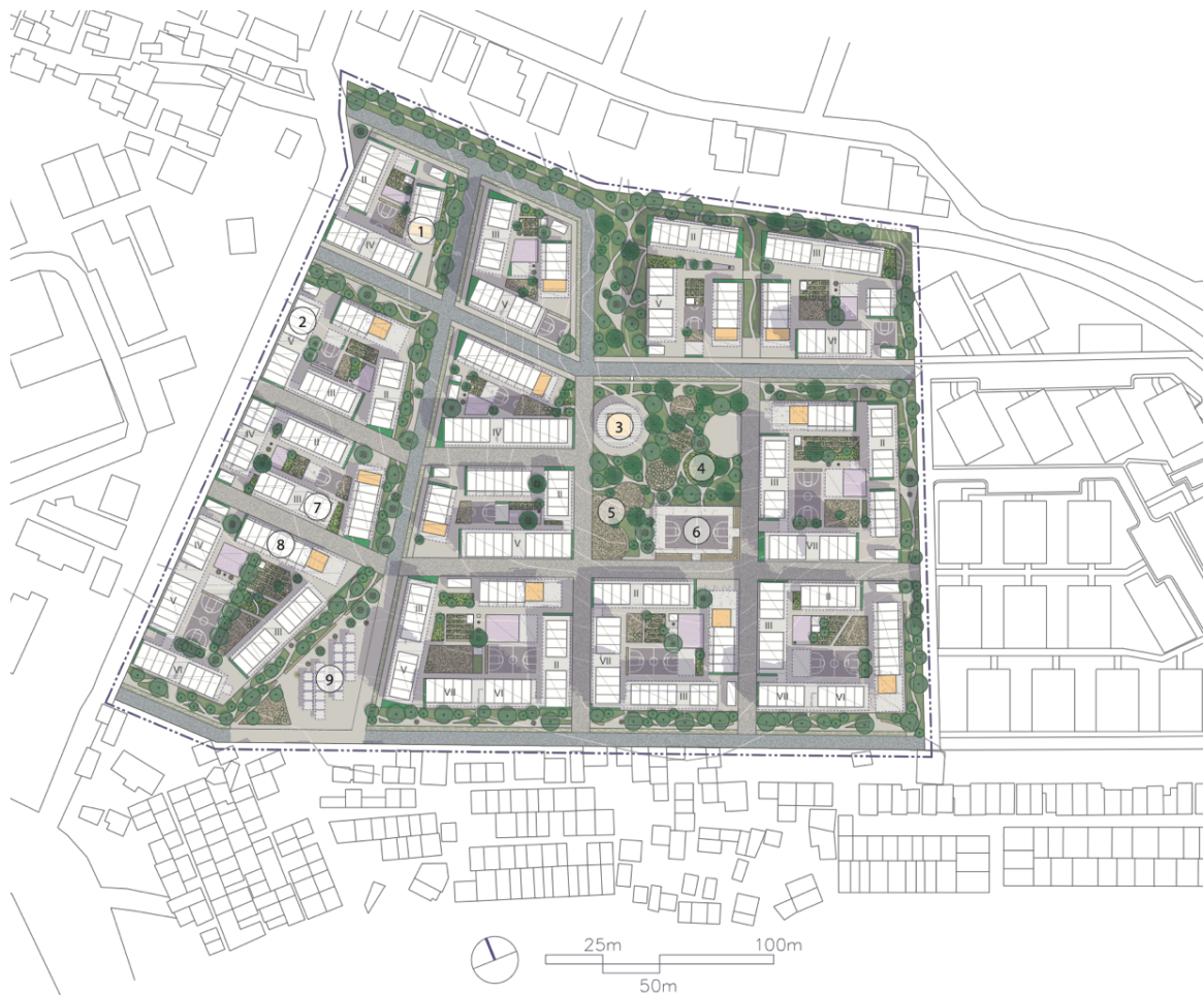
Figure 27. Masterplan showing proposal for entire site; 1 – block community building, 2 – five story rental unit building, 3 – neighborhood community center, 4 – shared urban gardening lot, 5 – playscape, 6 – Multipurpose roofed space with basketball court, 7 – three story lofted multifamily building, 8 – lofted rowhouse building, 9 – public square
