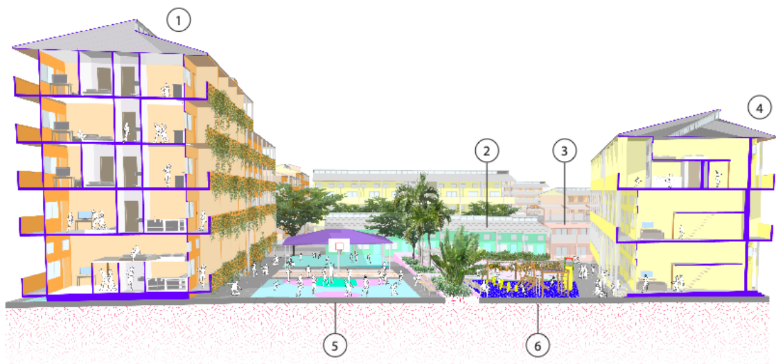
Figure 25. Section over courtyard; 1 - six story rental unit building, 2 - lofted rowhouse, 3 – block community building, 4 – three story lofted multifamily building, 5 – basketball court/open space for activities, 6 – playground (illustration credit Alexander Jones)
