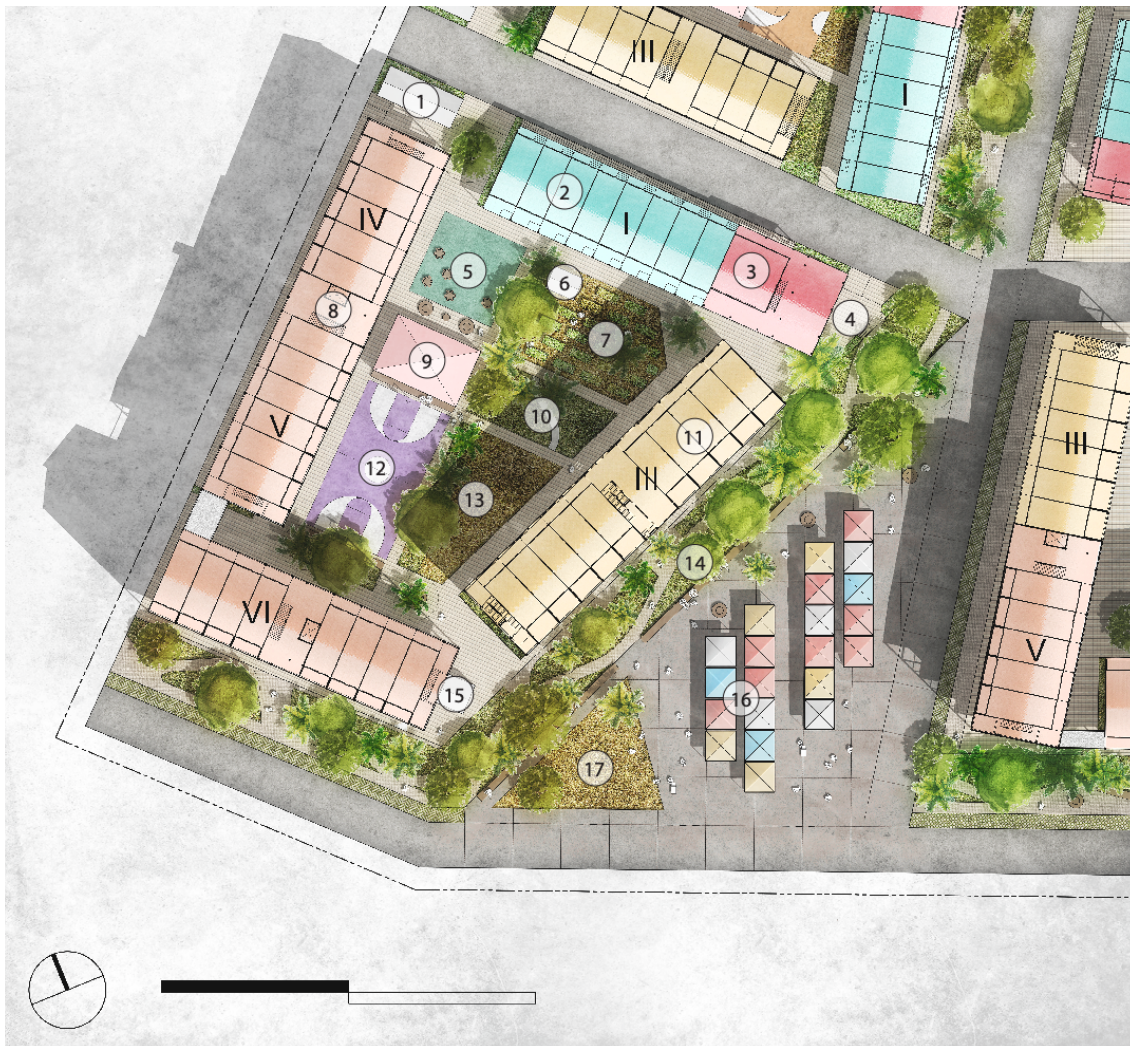
Figure 26. Zoomed plan of western corner of the site showing typical courtyard design and illustrated public place; 1- recycling station, 2 – lofted rowhouse building, 3 – community building, 4 – roofed outdoor space for local market or events, 5 – flexible space for dancing or seating, 6 – hen house, 7 – collective urban gardening, 8 – six story rental unit building, 9 – roofed multipurpose cultural space, 10 – forestry garden, 11 – three story lofted multifamily building, 12 – basketball court/open space for activities, 13 – playground, 14 – elongated park with green canopies, storm water collection, seating and pedestrian walk ways, 15 – workshop building, 16 – portable roofed market places, 17, public playground (illustration credit Brendan Cooney)
