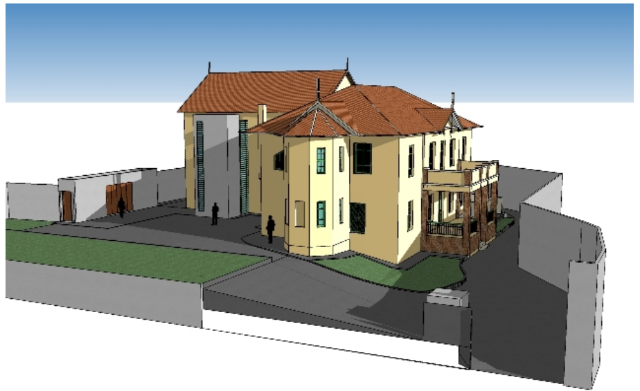
Figure 19: Model of the house viewed from the street, showing the structures to be added to the building, mainly the elevator tower (gray colored).
