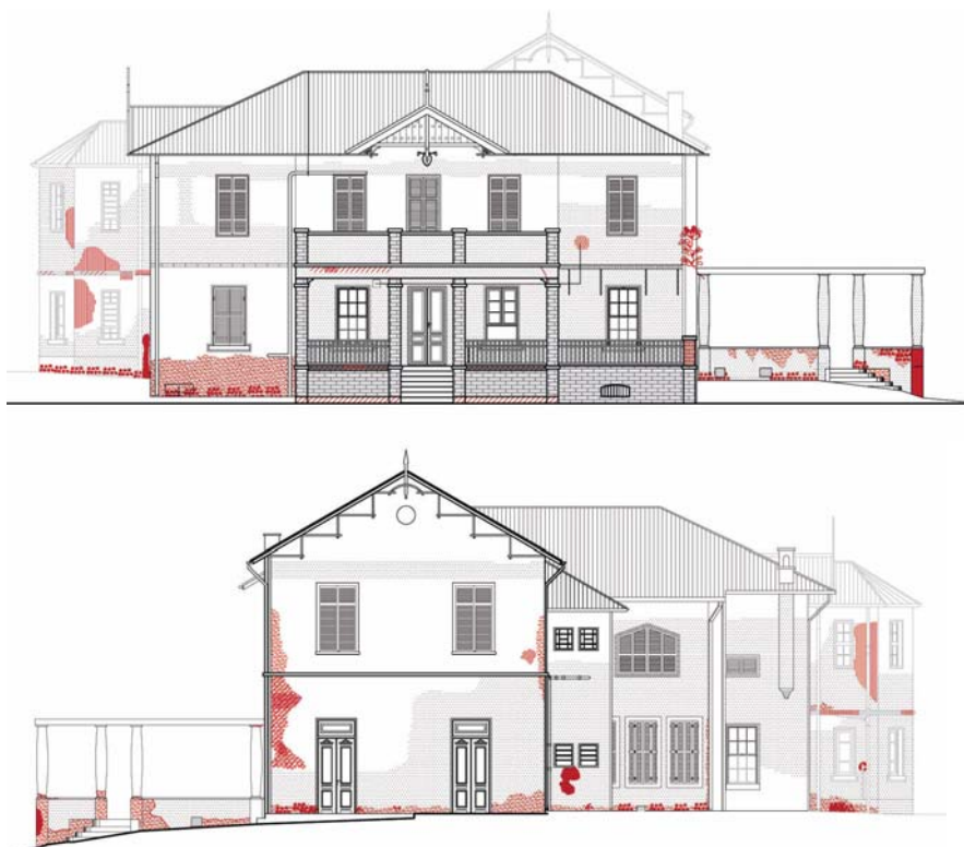
Figure 20, 21: North and South façades elevations, showing damaged paintings and plasters.
