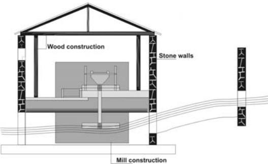
Fig 5. Technological scheme of Stolac mill
