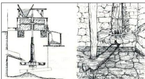
Fig. 4 Drawing of a horizontal water wheel, Marco Vitruvius Pollione
