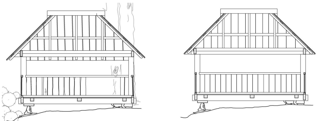
Longitudinal section, present condition and after conservation
