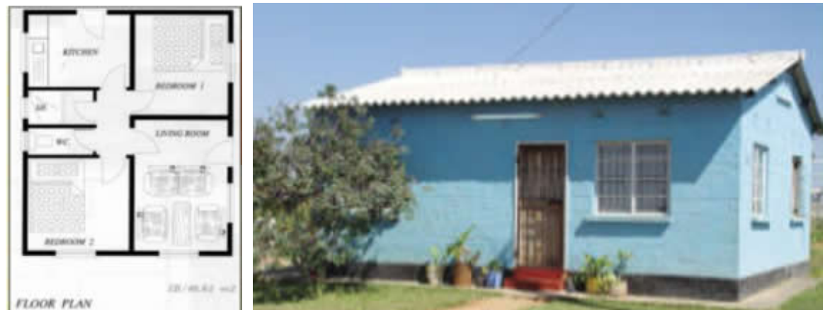
Fig 2: Floor plan and pictorial view of a 2004 NHA low cost house (source: NHA 2004)
