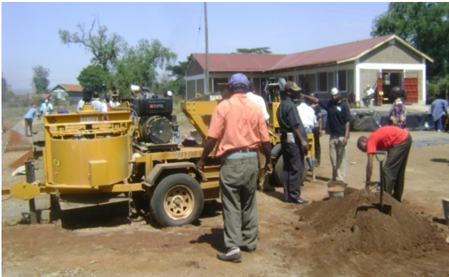
The Training of Ministry Housing Staff on ISSB Production at Nakuru ABT centre
