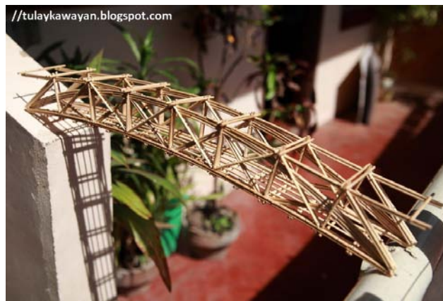
Figure 7 A scale model using barbecue stick and push pins to mimic the behaviour of bolt joints
